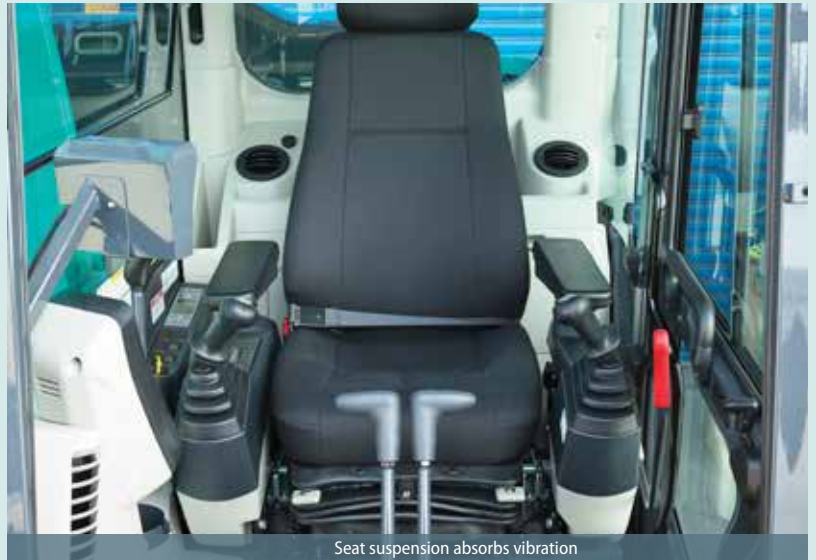
Seat suspension absorbs vibration
